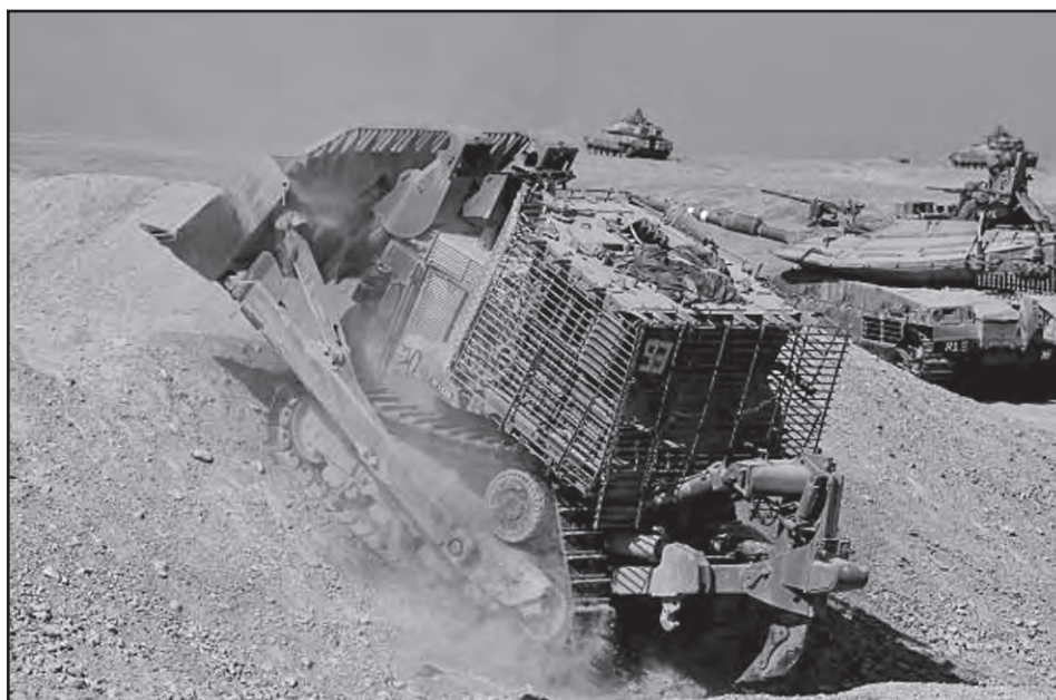
An Israel Defense Force (IDF) armored Caterpillar D-9 bulldozer clearing the way for IDF’s Mark IV main battle tanks.
